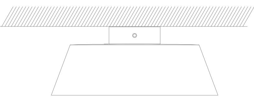
**Notes:** Do not energize luminaire until installation is completed. General contractor is responsible for providing appropriate anchoring devices to support load of fixture.
